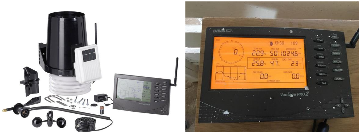
Figure 3. Automatic weather station (Davis Instruments Vantage Pro 2 DAV-6152EU, CA) used during experiment
